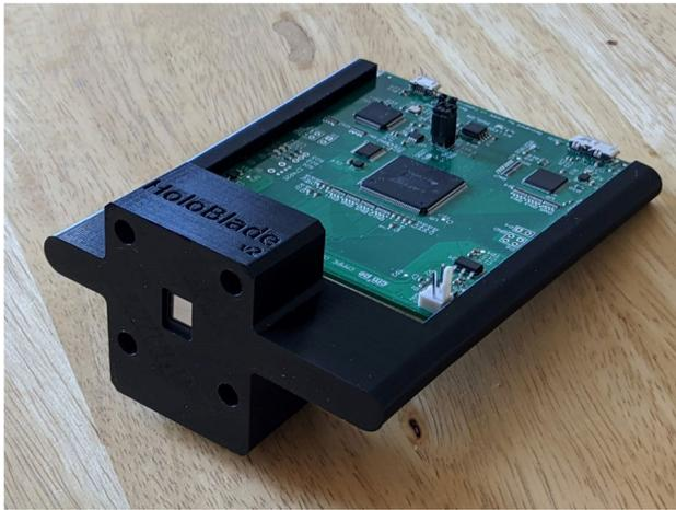
**Fig. 1.** HoloBlade, an open-hardware SLM driver-stack.
